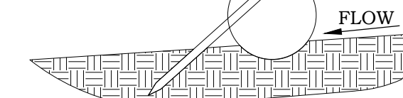
FIELD INSTALLATION USING STRAW OR WOOD FIBER
